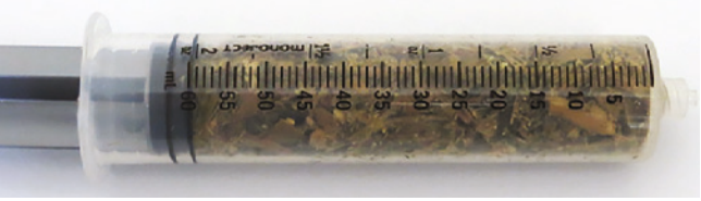
Figure 1: Example of gas-filled porosity for 30 g of corn silage (35 percent DM) in syringe at 60 cc.
