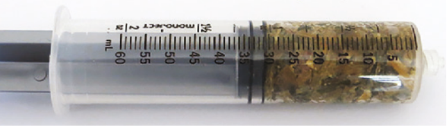
Figure 2: Example of gas-filled porosity for 30 g of corn silage (35 percent DM) in syringe compressed to 30 cc.
